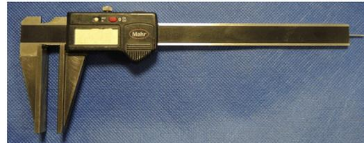
In general, measure the diameter of the wire rope at each WTG tower platform, and under the service lift, where the wire rope is less loaded. Specifically, if a wire rope wear is detected, measure on the affected area.
