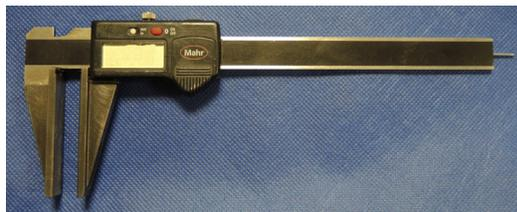
In general, measure the diameter of the wire rope at each WTG tower platform, and under the service lift, where the wire rope is less loaded. Specifically, if a wire rope wear is detected, measure on the affected area.
