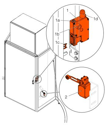
Figure 8: Guard locking system
