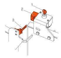
Figure 7: Trapped-key system
