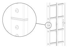
Figure 6: Gap between ladder sections
