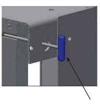
Overload adjustment tool (2) with security Torx 40
