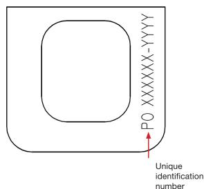
After installation, marking shall be completely accessible; otherwise additional marking near the anchor device will be necessary.
