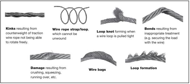
Figure 10: Wire rope damage examples
