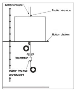
Figure 2: Securing the traction wire rope
